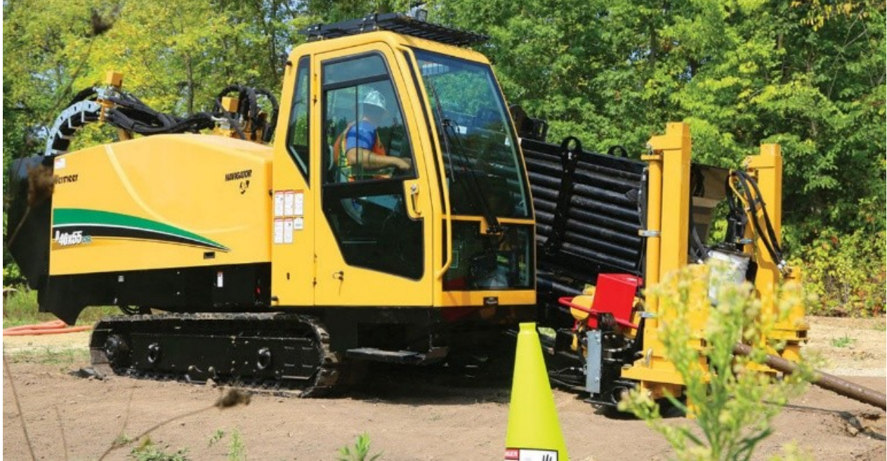
Figure 5. Vermeer horizontal directional drill (HDD) equipment used to place underground conduit
