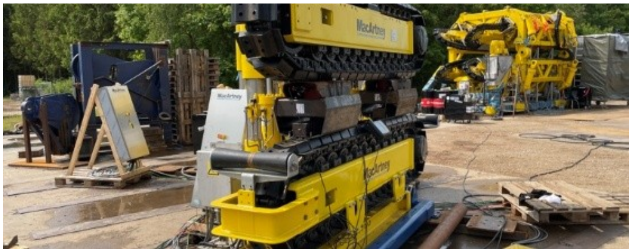
Figure 4. CEMAC cable offshore track tensioner used to cable tension with specification limits
